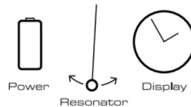
First, you need a device that can produce a periodic phenomenon (for example, a pendulum). This is the RESONATOR. Next you'll have to sustain the periodic motion by feeding it POWER
